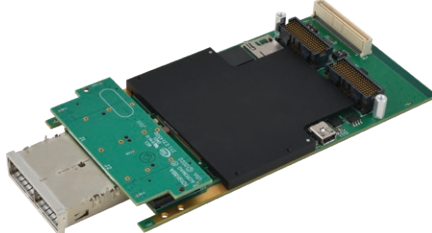
Above: XMC-FZU board shown with optional AXM plug-in I/O expansion module; At left: AXM-FZU01 I/O breakout board.
