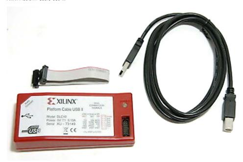
The XMC-7 Series FPGA mezzanine board is hosted on a carrier. To program the on-board FPGA, you will need to attach the JTAG cable to the carrier's 14-pin JTAG connector, then turn the host's power ON. Connect the USB cable from the JTAG programmer to the PC running Vivado. Once the JTAG programmer is recognized, locate and run Vivado.
