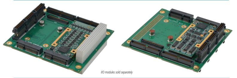
Two AcroPack or mPCle mezzanine module slots ◆ Non-Intelligent carrier card ◆ PCI/104-Express / PCIe/104 interface
