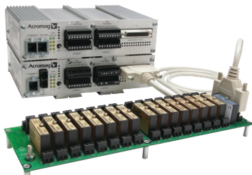
Interface to 8B signal conditioning modules.
