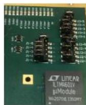
Figure 2: Jumper and LED Locations
