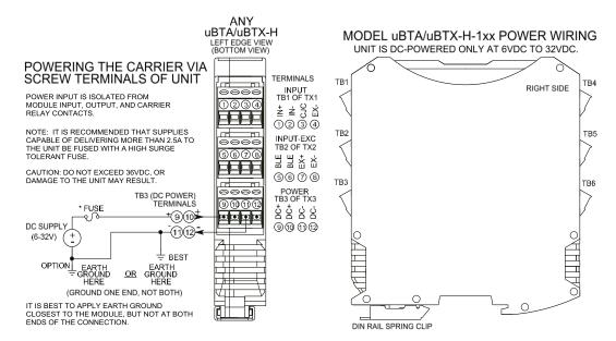
The unit may be optionally powered (or redundantly powered) via its DIN rail connector as shown below (optional terminal is required). The bus power connector of the module can be used to interconnect between modules by plugging them together and then connecting them as a group to a suitable power supply using an optional left or right terminal block, 1005-220 or 1005-221, as shown.
