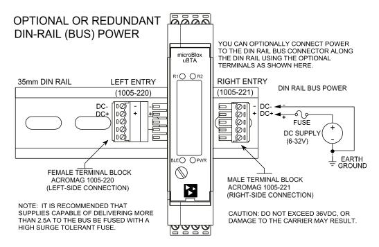
**IMPORTANT - Fusing:** It is recommended that supplies capable of delivering more than 2.5A of power to the carrier (or bussed carriers) be fused with a surge tolerant fuse. Unit includes a transient voltage suppressor clamp across its power input that will clamp transient overvoltage conditions. A sustained over-voltage condition from an unfused power supply could drive excessive fault current flow in the circuit that can damage the carrier if allowed to exceed 3A.
