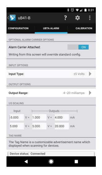
The screen at left is the uBTA Alarm configuration screen of the Agility mobile app. To configure a uB input module for installation in the alarm carrier, select the uBTA Alarm tab and drag the "Alarm Carrier Attached" switch right to ON as shown. Scroll down the page to complete the Alarm configuration.
