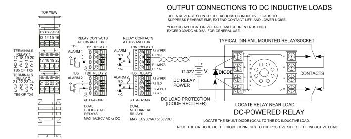
**IMPORTANT:** Because the solid-state relay of the uBTA-H-1SR model is <u>both</u> AC and DC rated, it is not possible to also include contact protection built-into the relay output of this device (a diode is normally used for DC, and a MOV for AC). The required protection is always best placed at the load as shown above. You should always include this protection in your installation when switching inductive loads, or damage to the relay could occur.
