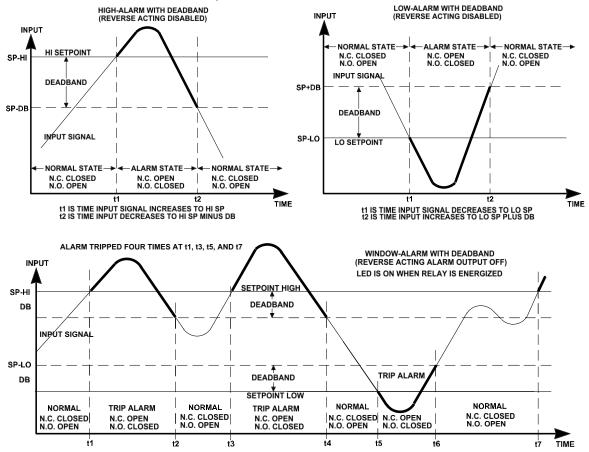
FOR THE WINDOW ALARM, THE ALARM IS TRIPPED WHEN THE INPUT SIGNAL IS OUTSIDE THE LOW & HIGH TRIP RANGES WITH DEADBAND APPLIED
