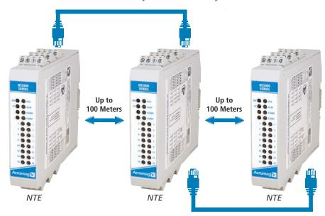
Connect NTE Ethernet I/O modules with a daisy-chain topology using the internal dual-port switch to simplify network cabling.
