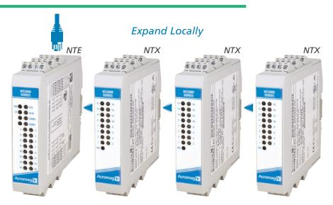
Link up to three NTX expansion I/O modules to an NTE Ethernet I/O module over the integrated DIN rail I/O bus connectors.
