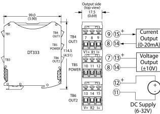
Dual channels ◆ Universal thermocouple, mV inputs ◆ 6-32V DC local/bus power
