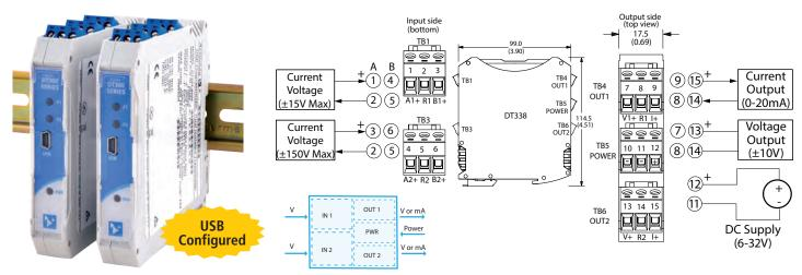
Dual channels ◆ ±15V, ±150V inputs ◆ 0-20mA, ±10V outputs ◆ 6-32V DC local/bus power
