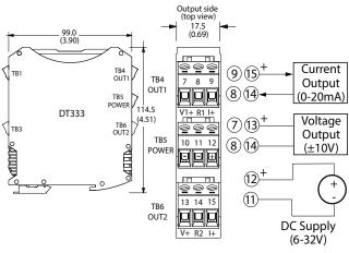
Dual channels ◆ Universal thermocouple, mV inputs ◆ 6-32V DC local/bus power
