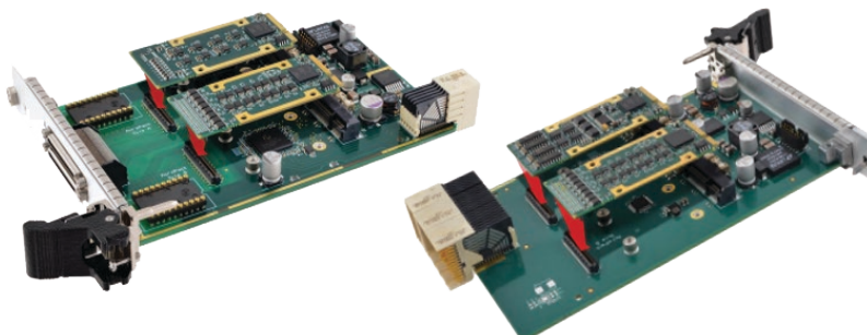
Figure 17: ACPS3310 (left) & ACPS3320 (right) Compact PCIe Serial
