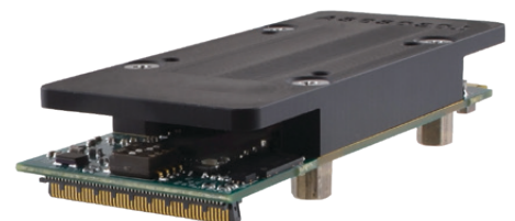
APZU-30x with included heat spreader attached
