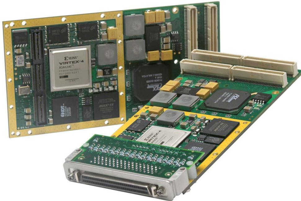
*Acromag FPGA PMCs shown with and without plug-in AXM I/O extension modules*
