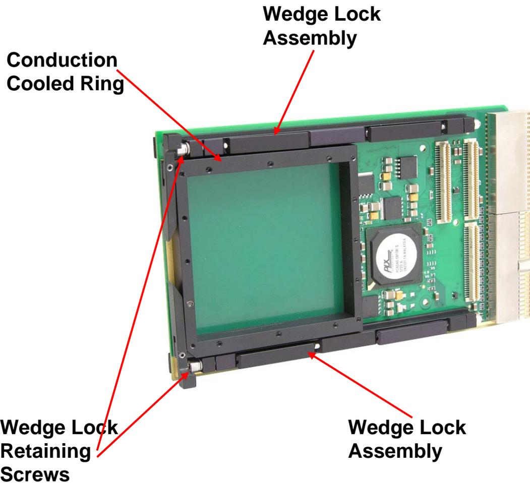
Acromag's [AcPC4610CC](#) 3U Compact PCI Conduction Cooled PMC Carrier Card.
