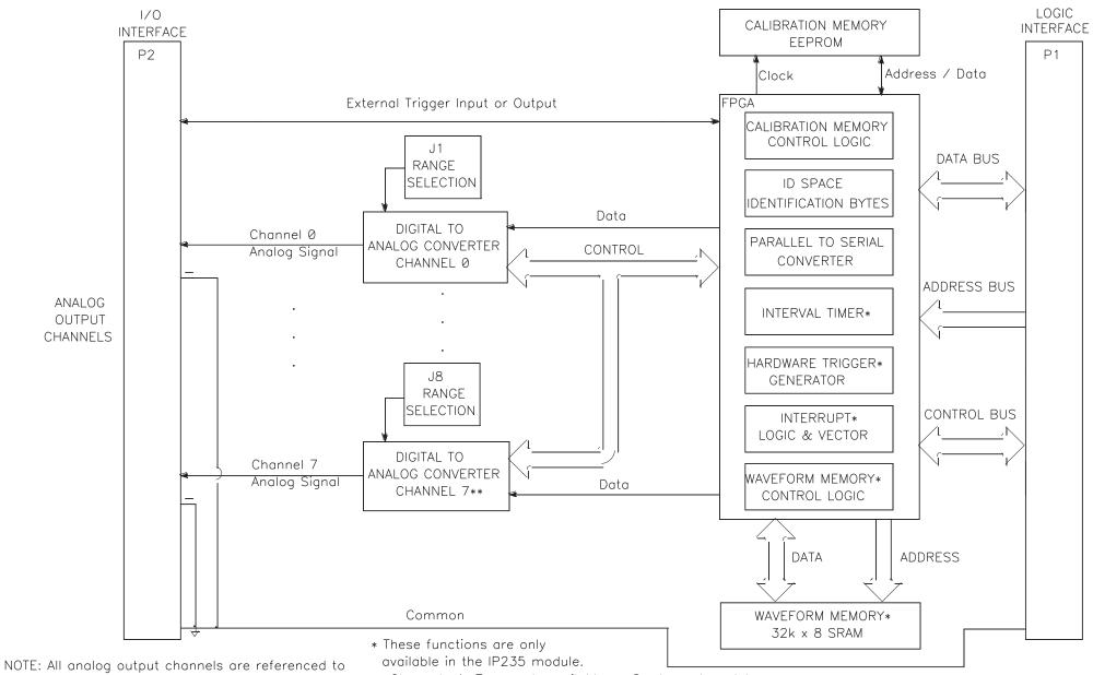
NOIE: All analog output channels are referenced to analog ground. To avoid ground loops do not connect grounded loads to the negative side of the output.
