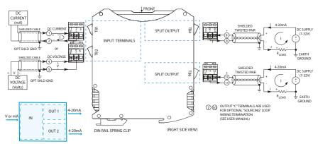
DC current and low voltage input ◆ 4-20mA outputs (sink/source) ◆ 7-32V DC loop power
