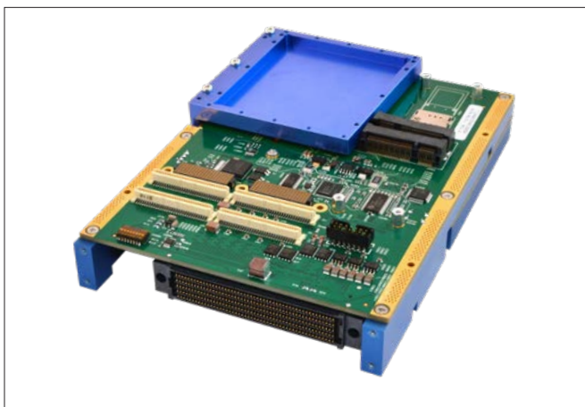
ACEX-4610 carrier card bottom view showing PMC/XMC slot
