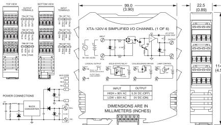
6 discrete input/output channels •
