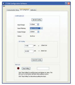
TT336 Model software allows you to configure transmitters offline, save the file, and download into units later, at your convenience.
