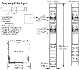
Multi-range frequency/pulse input ◆ 4-20mA output (sink/source) 12-32V DC local/local power
