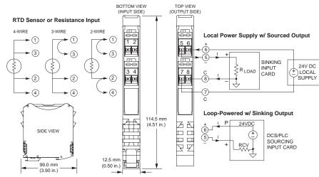
RTD (Pt, Ni, Cu) or 0-450 ohm input ◆ 4-20mA output (sink/source) ◆ 12-32V DC loop/local power
