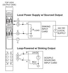
12-32V DC loop/local power 100 ohm Pt RTD or 0-900 ohm input ◆ 4-20mA output (sink/source) ◆
