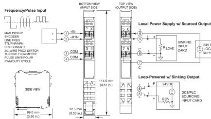
Multi-range frequency/pulse input ◆ 4-20mA output (sink/source)
