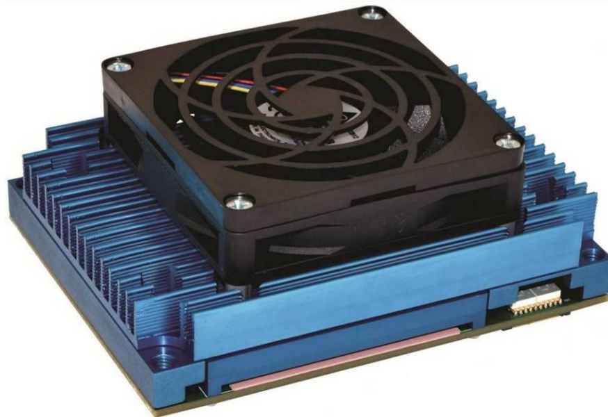
Fig. 3.14.5.e: XCOM-6400 with Heat Spreader and Active Heat Sink
