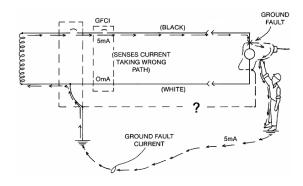
If the current returned in neutral does not match the current in the hot line, the GFCI will trip and interrupt the current flow out of the hot wire. Of course, the "lost" current doesn't really go "missing," but has temporarily found some other path back to the source, perhaps through yourself to earth. This errant path is the ground fault we refer to and the GFCI feeding this circuit will trip very quickly to prevent serious shock or electrocution via current in this errant path.
