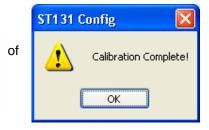
At this point, the transmitter is calibrated. Click OK to continue. Check the accuracy a few other points. Note that if your input type is Pt RTD, your output will be linear with the input temperature, not the input resistance.
