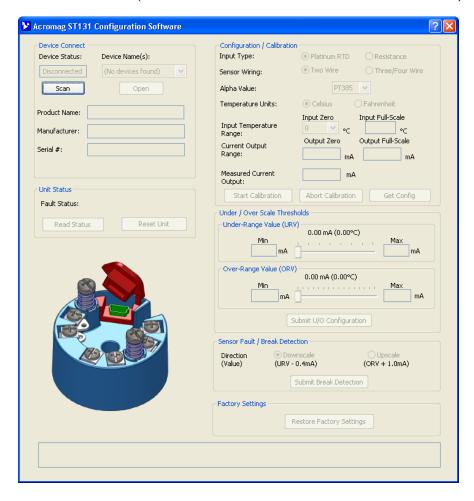
Note that without a device already connected via USB, the Device Status field indicates "Disconnected". After you connect USB, the first step to begin reconfiguration is to select the device to connect to using the scroll window of the Device Name field. Use the scroll bar to click on and select a transmitter from this list in order to open it for reconfiguration (use the serial number to discern a particular transmitter). Then click the "Open" button to connect to the selected device.
