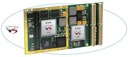
Download your own programs into the reconfigurable FPGA to quickly create custom I/O module. Optional I/O modules plug into the front mezzanine.
