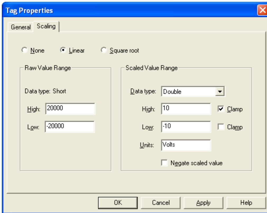
Tag scaling is optional and can be used to convert raw data from a device into engineering units. When the 914MB is using its default Input Configuration ( $\pm 10V$ ), a channel input value of  $-20000$  corresponds to  $-10V$  and a value of  $20000$  corresponds to  $10V$ . The following steps configure this scaling for the tag.
