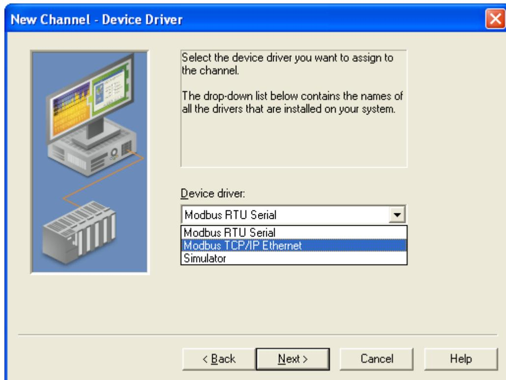
3. **Device Driver** – Select **Modbus TCP/IP Ethernet** from the drop-down menu.
