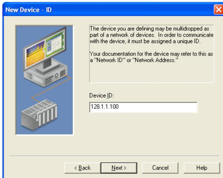
18. **ID** – Set the device ID to match the current TCP/IP ID of the I/O module. For example, if the module is in Default Communication mode, set the ID to 128.1.1.100.
