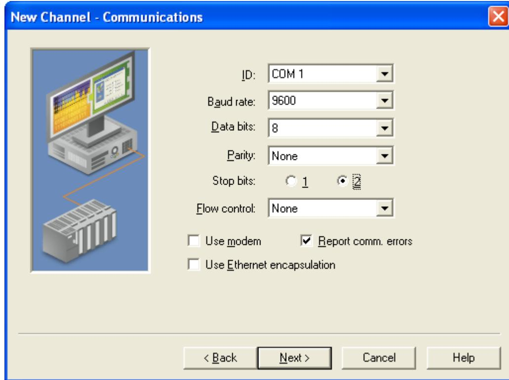
4. **Communications** – Set the communication parameters to match the current configuration of the I/O module. For example, if the module is connected to COM port 1 and is in Default Communication mode, make the following selections:
