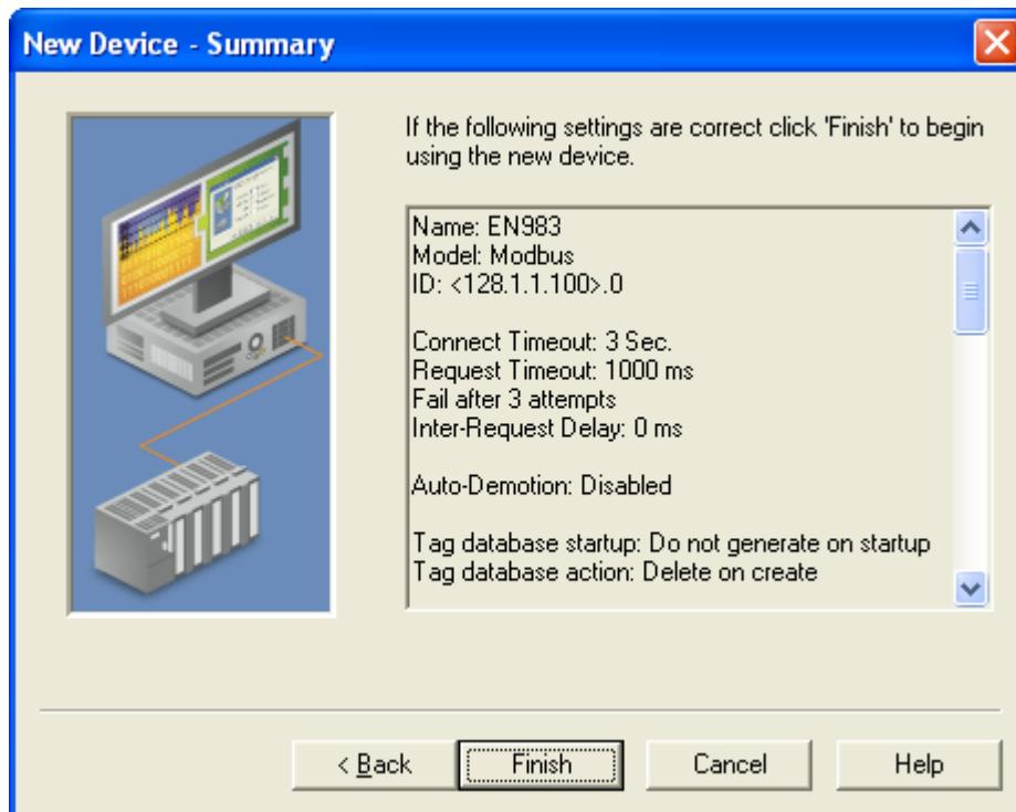
28. **Summary** – This page summarizes the selections made on the previous pages. Click **Finish** to exit the wizard and add the device to your project. A device icon will be added to the **Channel Device Group** area of the main program window. Settings for the device can be modified in the future by right clicking on the device icon and selecting **Properties...**
