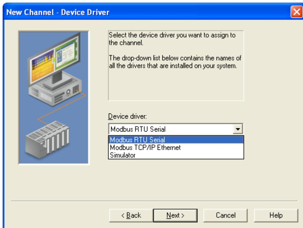
3. **Device Driver** – Select **Modbus RTU Serial** from the drop-down menu.
