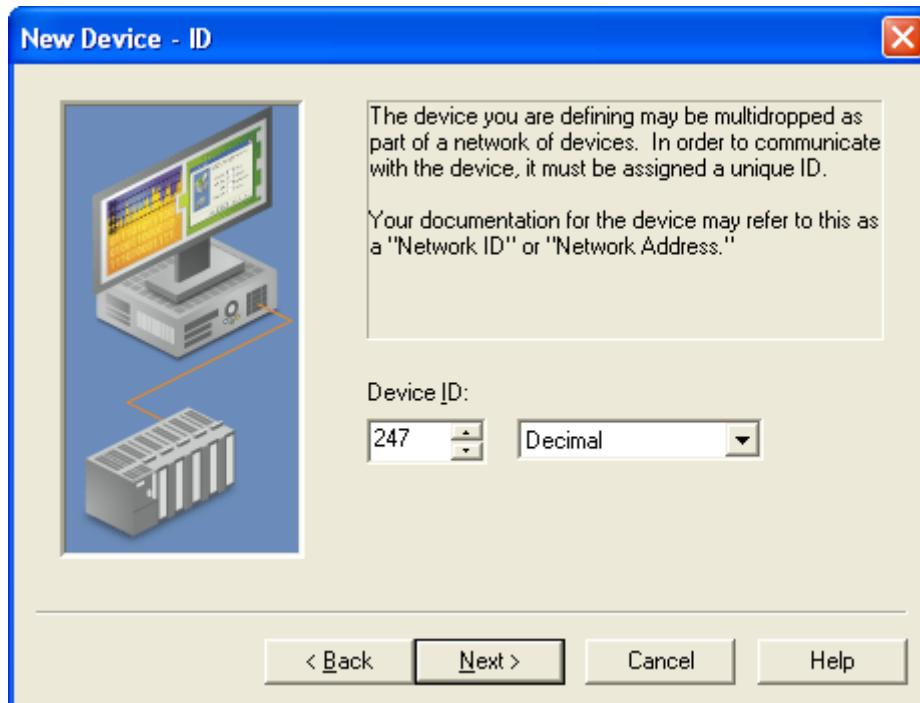
4. **ID** – Set the device ID to match the current Slave Address of the I/O module. For example, if the module is in Default Communication mode, set the ID to 247.
