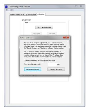
**NOTE:** To measure current, you can alternatively connect a voltmeter across a precision load resistor, and then accurately read the output current as a function of the IR voltage drop produced in the resistor (recommended for current outputs).
