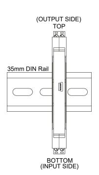
TILT MODULE UPWARD TOWARDS RAIL AND HOOK ONTO UPPER LIP OF RAIL. ROTATE MODULE DOWNWARD TO ENGAGE SPRING CLIP ONTO LOWER LIP OF RAIL.
