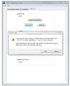
Once you've configured the transmitter, you are ready to install it in the field, as the transmitter has already been factory calibrated. If you later encounter error that is out of specification, you can click the "Calibration" tab to display the Calibration control page shown at left.
