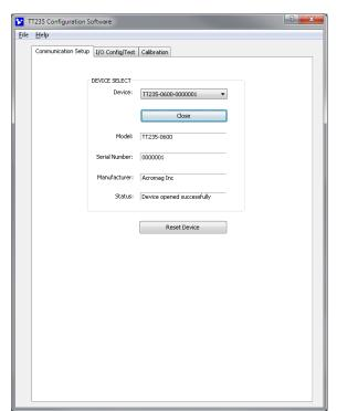
Select a transmitter from the drop down menu. When you click on a transmitter name from the drop down menu, the software will automatically attempt to open a connection with the selected transmitter. If the software does not have an open connection with the transmitter, click the **[Open]** button to open a connection with the transmitter.
