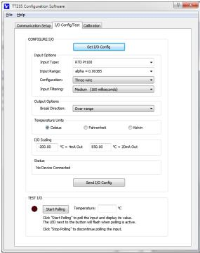
At this point, you can click the "I/O Config/Test" tab to begin configuring the transmitter, or to optionally test its operation. The I/O Config/Test window is the second image shown at left.
