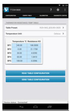
This transmitter can be configured and calibrated via the Acromag Agility™ Config Tool App. This software can be downloaded free of charge from the Google Play store at <u>play.google.com</u>. To connect to this transmitter, a USB OTG (On-The-Go) cable (Acromag 5028-565) and USB A to Mini-B cable (Acromag 4001-113) are required. This app is compatible with Android devices using Ice Cream Sandwich (4.0) or later.
