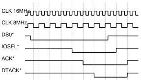
Note that the select line (IOSEL\*, IDSEL\*, MEMSEL\* or INTSEL\*) is held active a short time after DTACK\* is issued. However, the IP module should not expect data to be held after ACK\* is detected by the carrier board in a data write cycle.
