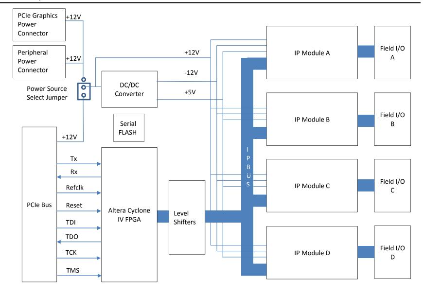
Figure 1 APCe8650 Block Diagram
