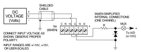
Connect input voltage to input positive (+) and negative (-) while observing proper polarity. If the input source is floating, it is recommended that you connect the negative input to the analog common terminal of the port (terminal C). Additionally, analog common (C) should also be connected to earth ground at one point.
