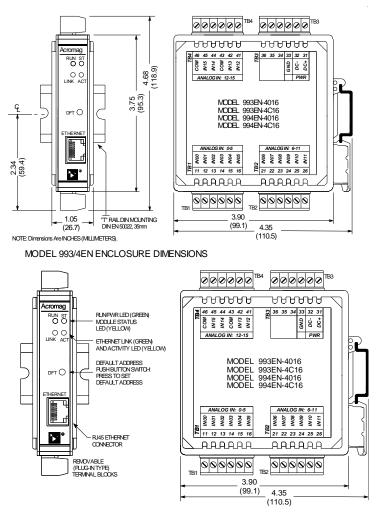
The front panel DFT push-button is used to toggle the module into or out of Default Mode. In Default Communication Mode, the module assumes a fixed static IP address of "128.1.1.100", a default subnet mask of "255.255.255.0", a default username of "User", and a default password of "password00". To activate, depress the DFT button for 5 seconds, until the ST LED blinks on/off slowly. To disable, depress the DFT button for 5 seconds or until the ST LED stops blinking.
