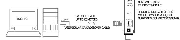
Refer to the Accessory Cables section at the back of this manual for more information on accessory cables including patch and crossover cables available from Acromag and other vendors.
