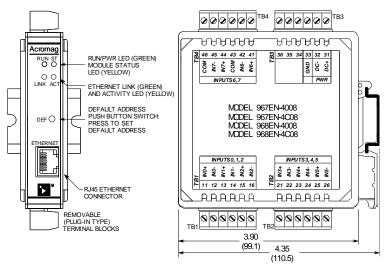
The front panel DFT push-button is used to toggle the module into or out of Default Mode. In Default Communication Mode, the module assumes a fixed static IP address of "128.1.1.100", a default subnet mask of "255.255.255.0", a default username of "User", and a default password of "password". To activate, depress the DFT button for 5 seconds, until the ST LED blinks on/off slowly. To disable, depress the DFT button for 5 seconds or until the ST LED stops blinking.
