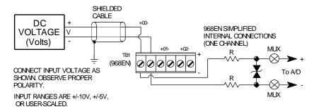
Connect input voltage to input positive (+) and negative (-) while observing proper polarity. If the input source is floating, it is recommended that you connect the negative input to the analog common terminal of the port (terminal C). Additionally, analog common (C) should also be connected to earth ground.
