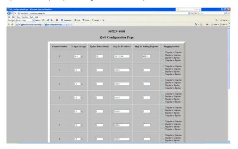
This unit has 1 port of 8 input channels of current (967EN), or voltage (968EN). For simplicity, the bipolar analog I/O channels of BusWorks modules are all normalized to ±20000 counts, representing ±100%. Likewise, BusWorks unipolar channels are normalized to 0-20000, representing 0-100%.
