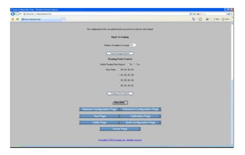
These models have eight input channels of current (967EN), or voltage (968EN). The Input Configuration page of the 968EN voltage unit is shown above. The 967EN is identical, except that it refers to current ranges.
