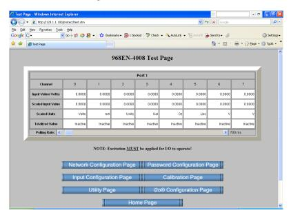
**Voltage or Current Inputs:** Note that the 8 input channels of these modules are grouped into one port. If the channel is not configured for floating point, which is necessary to accomplish scaling and totalizing, then "Inactive will be indicated for the scaled input value, scaled units, and Totalized value.
