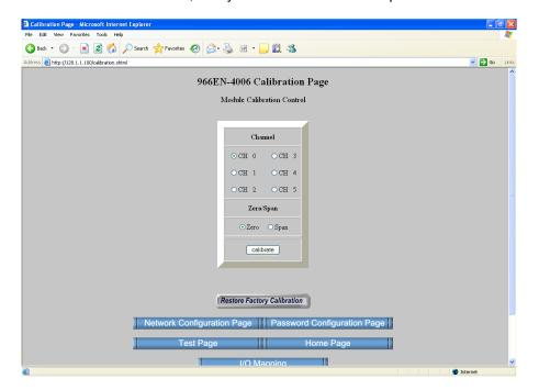
Note that if calibration has been done improperly at any input, you may click on the **Restore Factory Calibration** button to return the module to its original factory calibration for <u>all</u> channels.
