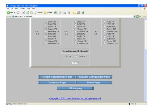
**IMPORTANT:** The input signal indicated only reflects the level of the inputs at the moment this screen is invoked and this does not continuously update. You can click your browser's refresh button to get a new input update.
