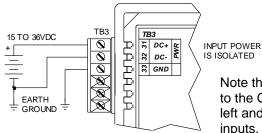
Note that earth ground is connected to the GND terminal as shown at left and is not connected to the inputs.
