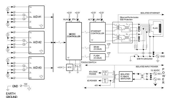
Note that input types may vary between channel pairs, but pair members share the same input range configuration—channel 0 and 1 may be configured differently from channel 2 and 3, and channel 4 and 5. All inputs share the same break detect direction, upscale or downscale. Inputs are not isolated channel-to-channel.
