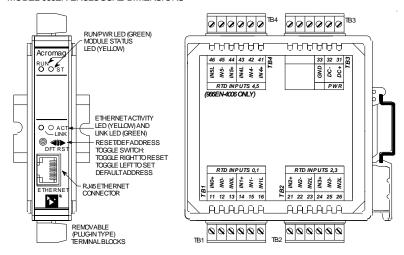
The toggle switch is used to toggle the module into or out of Default Mode (toggle left), or to reset the module (toggle right). In Default Communication Mode, the yellow ST LED blinks slowly and the module assumes a fixed static IP address of "128.1.1.100", a default subnet mask of "255.255.255.0", a default username of "User", and a default password of "password00".
