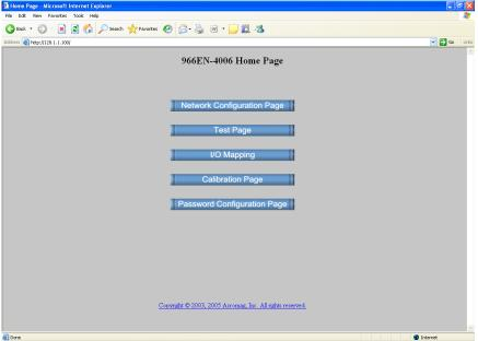
The Home Page provides buttons to access the other web pages of this module that are used to configure network parameters, change the user name and password, calibrate the module, map inputs to outputs, and operate/test the module.
