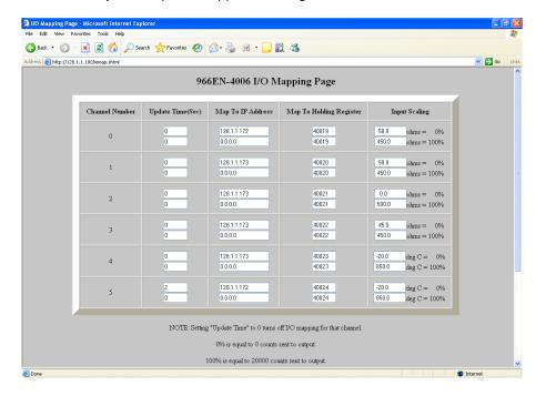
You can map each input channel to one or two analog output channels of another 972EN or 973EN module. The Map To Holding Register determines the output channel it will map to. Since the input signal is in wide-range engineering units, you must also specify the scaling between the input units and 0-100% at the output channel.
