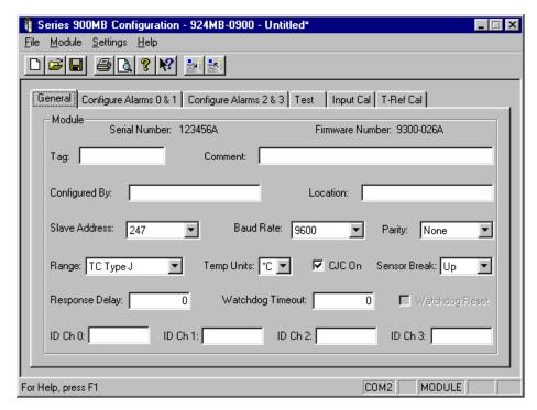
Use the "Parity" scroll bar to select Odd, Even, or No Parity (Default Mode) error checking by the module.
