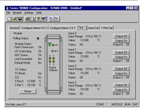
Keep in mind that alarm control of the output has priority over direct control (if enabled) and will seek to maintain the correct output state relative to the input level each time the input is scanned.
