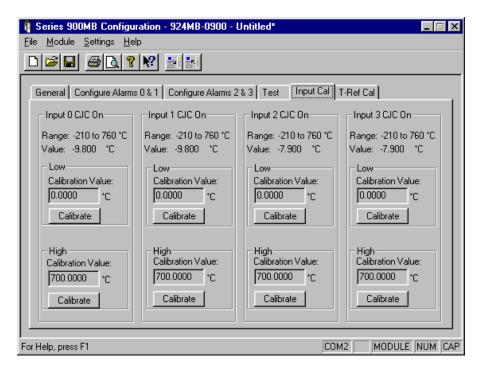
After upload, the Low and High calibration values will then be indicated in the Calibration Value fields. Uploading first will help prevent miscalibration if the input range set at the module is different than that selected via this software.
