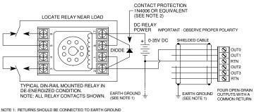
NOTE 1: RETURNS SHOULD BE CONNECTED TO EARTH GROUND AT THE SAME POINT TO AVOID CIRCULATING GROUND CURRENTS. NOTE 2: DIODE ADDED LOCAL TO INDUCTIVE LOAD TO SHUNT THE REVERSE EMIT THAT IS GENERATED WHEN CURRENT THROUGH THE INDUCTOR (RELAY COIL) IS TURNED OFF.
