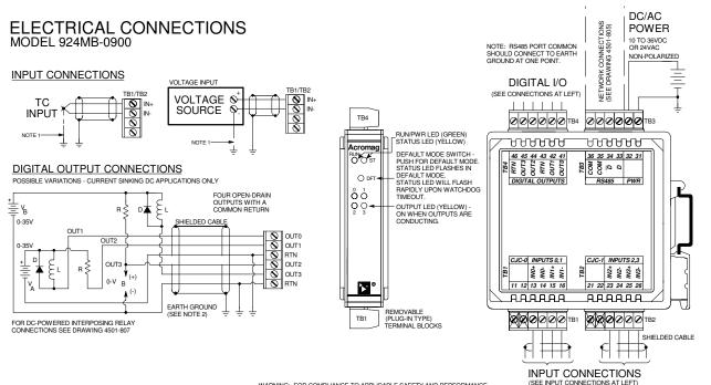
NOTE 1: THIS GROUND CONNECTION IS RECOMMENDED FOR BEST RESULTS. IF SENSORS ARE INHERENTLY CONNECTED TO GROUND, USE CAUTION AND AVOID MAKING ADDITIONAL GROUND CONNECTIONS WHICH COULD GENERATE GROUND LOOPS AND MEASUREMENT ERROR. NOTE 2: RETURNS SHOULD BE CONNECTED TO BATH GROUND AT THE SAME POINT TO AVOID CIRCULATING GROUND CURRENTS. NOTE 3: EXTERNAL PULLUP RESISTOR (USER SUPPLIED).
