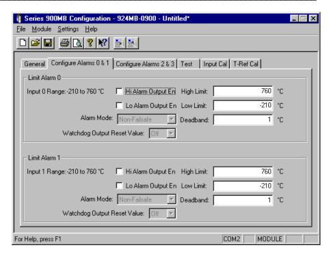
Deadband is normally used to eliminate false trips or switch "chatter" caused by fluctuations of the input near the limit.
