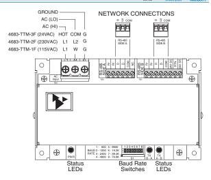
For N2 or BACnet MS/TP bus ◆ Drives up to 32 RS-485 devices ◆ Isolates and boosts signal up to 4000 ft.
