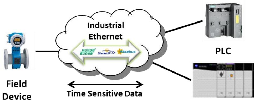
All of this activity on the network is a “necessary evil” and can dramatically influence the response of the field device. This activity can be so overwhelming for devices that time sensitive data stops being managed by the device. The following sections describe the different types of network activities and explain how PriorityChannel provides a device with immunity from this activity.
