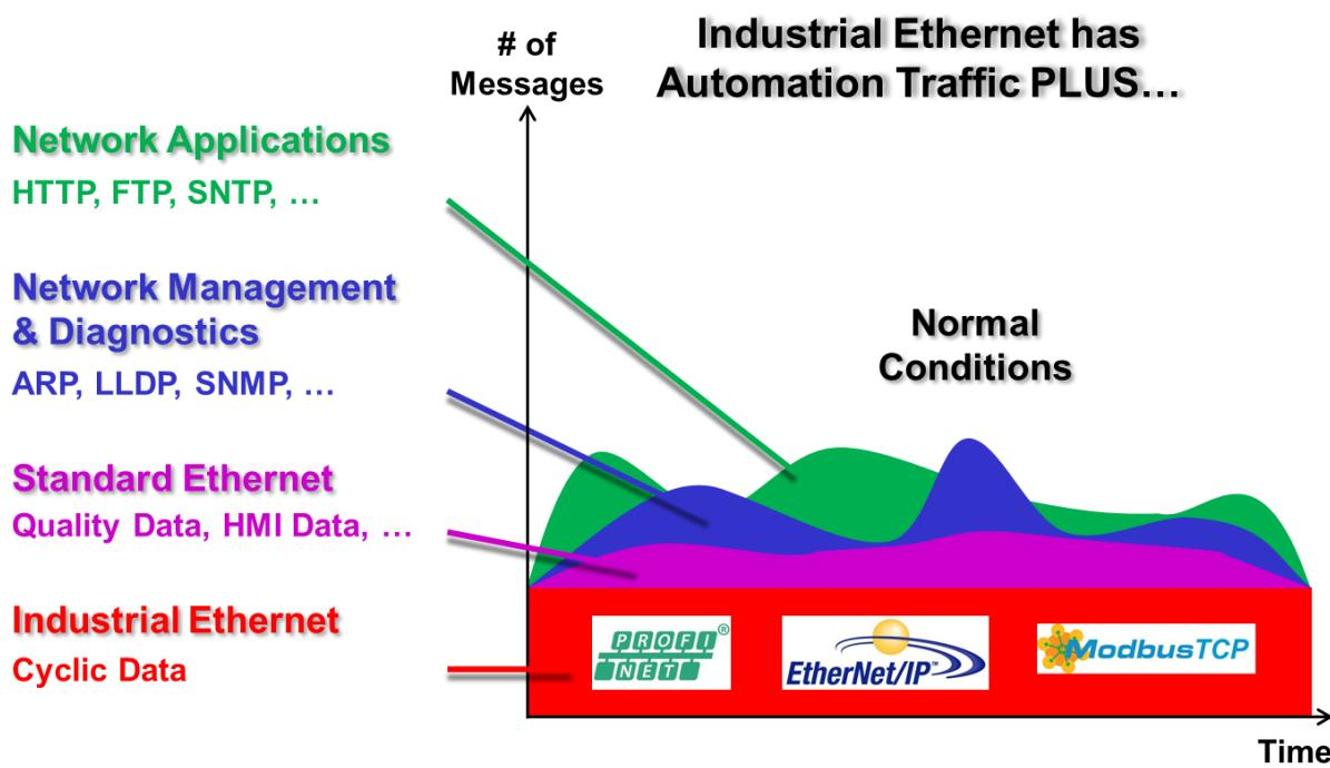
Standard Ethernet traffic is from other non-automation applications out on the wire and in the end device. This can be data destined for a printer from an HMI device on the network, or quality data destined for the front office. Typically, standard Ethernet traffic is minimized on the factory floor.
