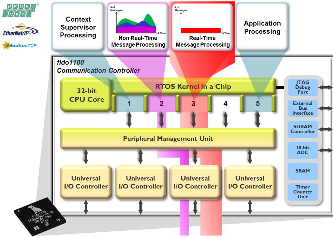
In traditional architectures, the TCP/IP stack is a non-re-entrant thread so it must be processed to completion even if the application has a higher priority message ready for processing. This means an ARP message, for example, will complete its processing by the TCP/IP stack even if it is time for the field device application to get its data to the PLC. If the PLC requires this data at a 2 ms rate, for example, it may arrive at 2 ms one time and 3 ms
