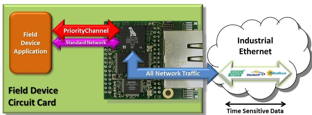
It is important to point out that PriorityChannel is not just fancy filtering. While certain message types are handled by the switch, most messages are passed to the communication controller – in this case, the Innovasic fido1100. There, the messages are identified so message
