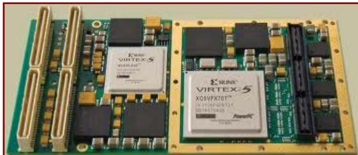
**Acromag FPGA PMC card** enables reconfigurable high performance I/O processing and user-customizable computing for video, 3D data, radar/sonar, software-defined radio, electronic warfare, floating-point math and fuzzy logic algorithm applications.
