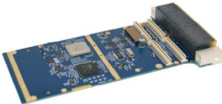
The board interconnects are high speed MultiGIG RT connectors from Tyco. These new high speed connectors allow for the use of high speed serial buses upwards of 10 Gbps and beyond.
