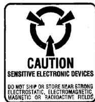
The board utilizes static sensitive components and should only be handled at a static-safe workstation.
