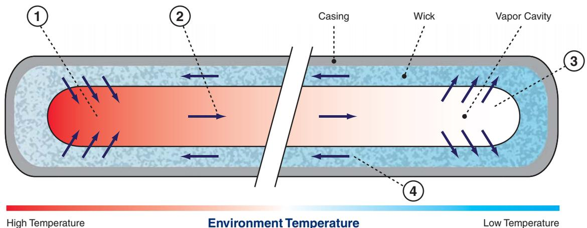
**Heat Pipe Thermal Cycle**
