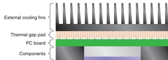
*Figure 4: Cooling fins dissipate heat from the board*
