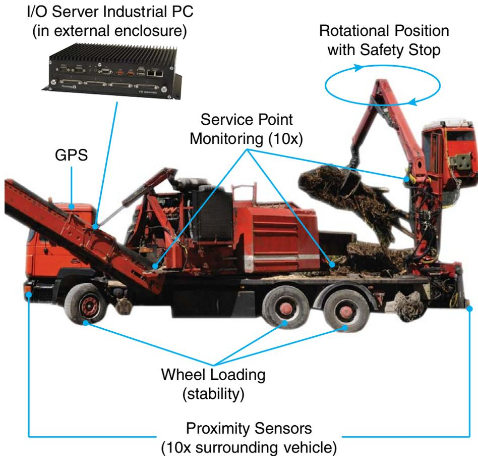
Commercial WiFi dongles and GPS antennae/receivers are used to keep system costs down and to take advantage of the manufacturer-provided software drivers. Two high-retention USB ports help keep the devices securely in place.
