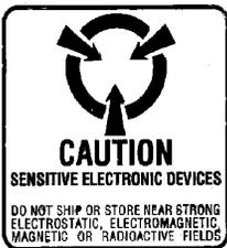
This board is physically protected with packing material and electrically protected with an anti static bag during shipment. It is recommended that the board be visually inspected for evidence of mishandling prior to applying power.
