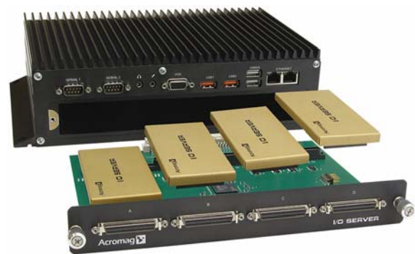
Figure 3: I/O modules on an integrated carrier
